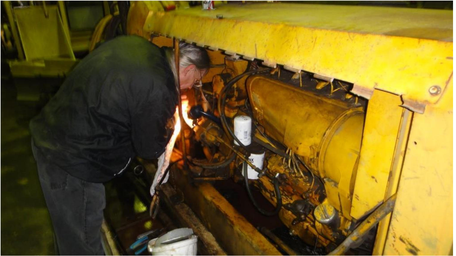
Fred installs a new fuel pump on the rail-mounted air-compressor
