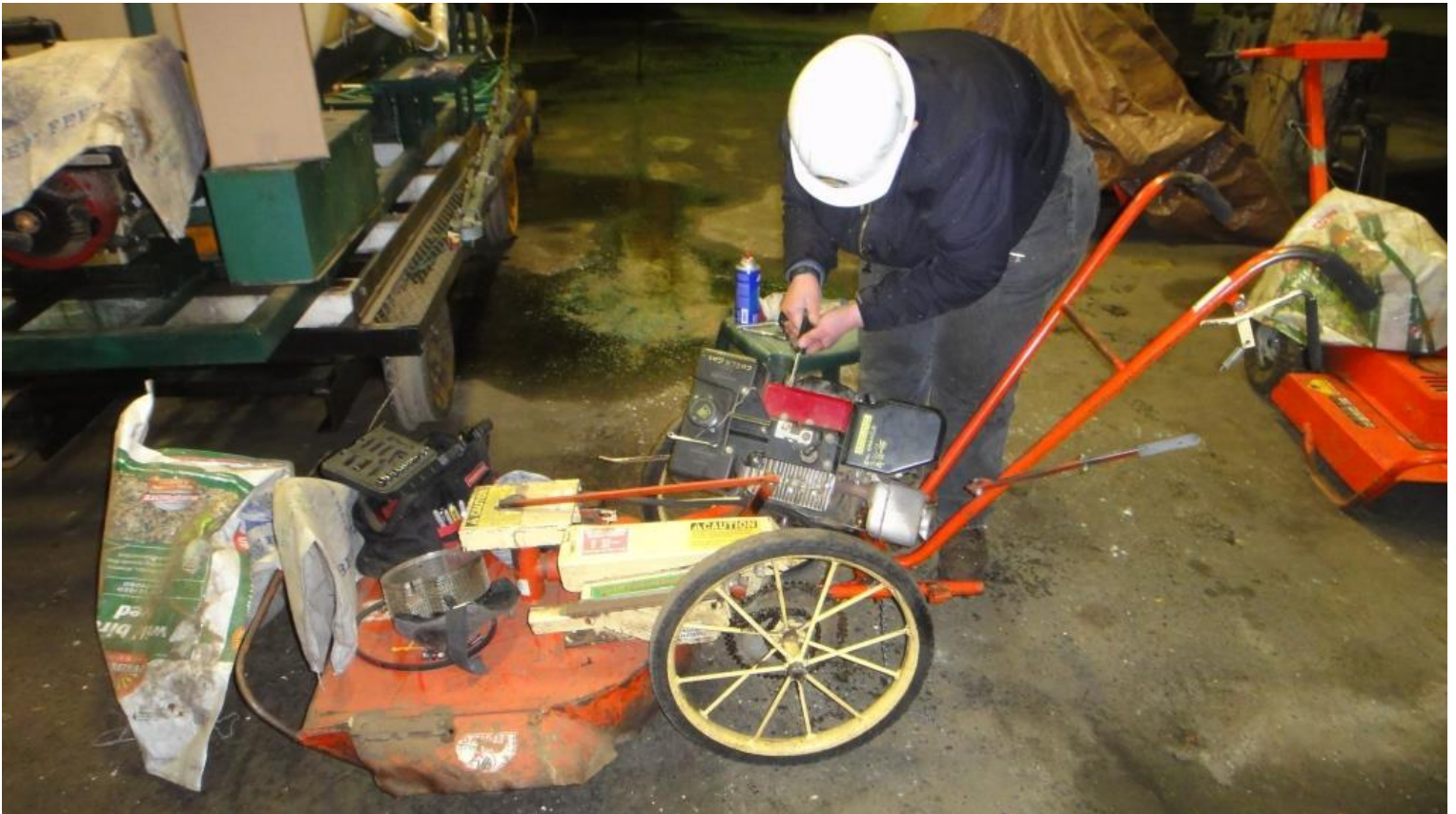
Heather installs a new clutch on the field-and-brush mower
