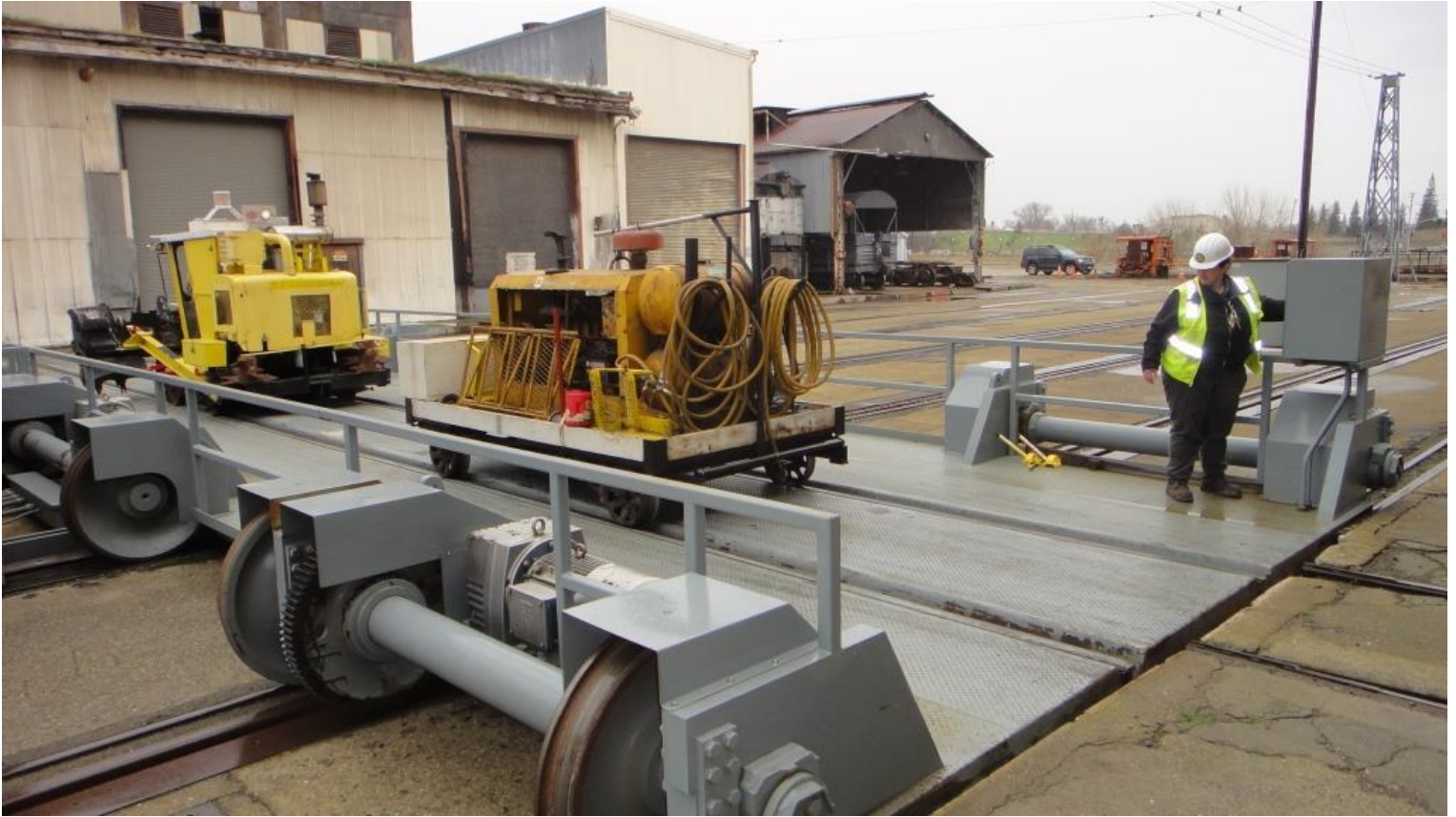
Heather at the controls of the transfer-table handles switching-out the compressor for the scarifier
