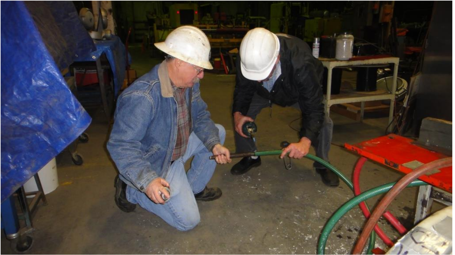
In order to re-plumb the 65-gallon spray-rig, Mike H. and Fred heat the hose to make it fit on the fitting
