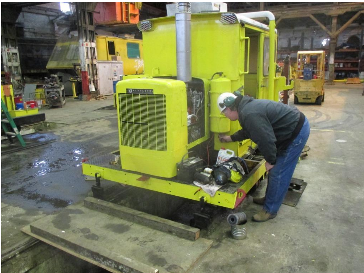
Chris installs a drain valve on the Kalamazoo's air tank
