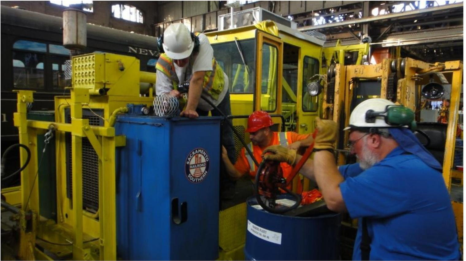
Steve fills the new-old tamper's hydraulic tank while Frank pumps hydraulic fluid and Joe checks the gauge
