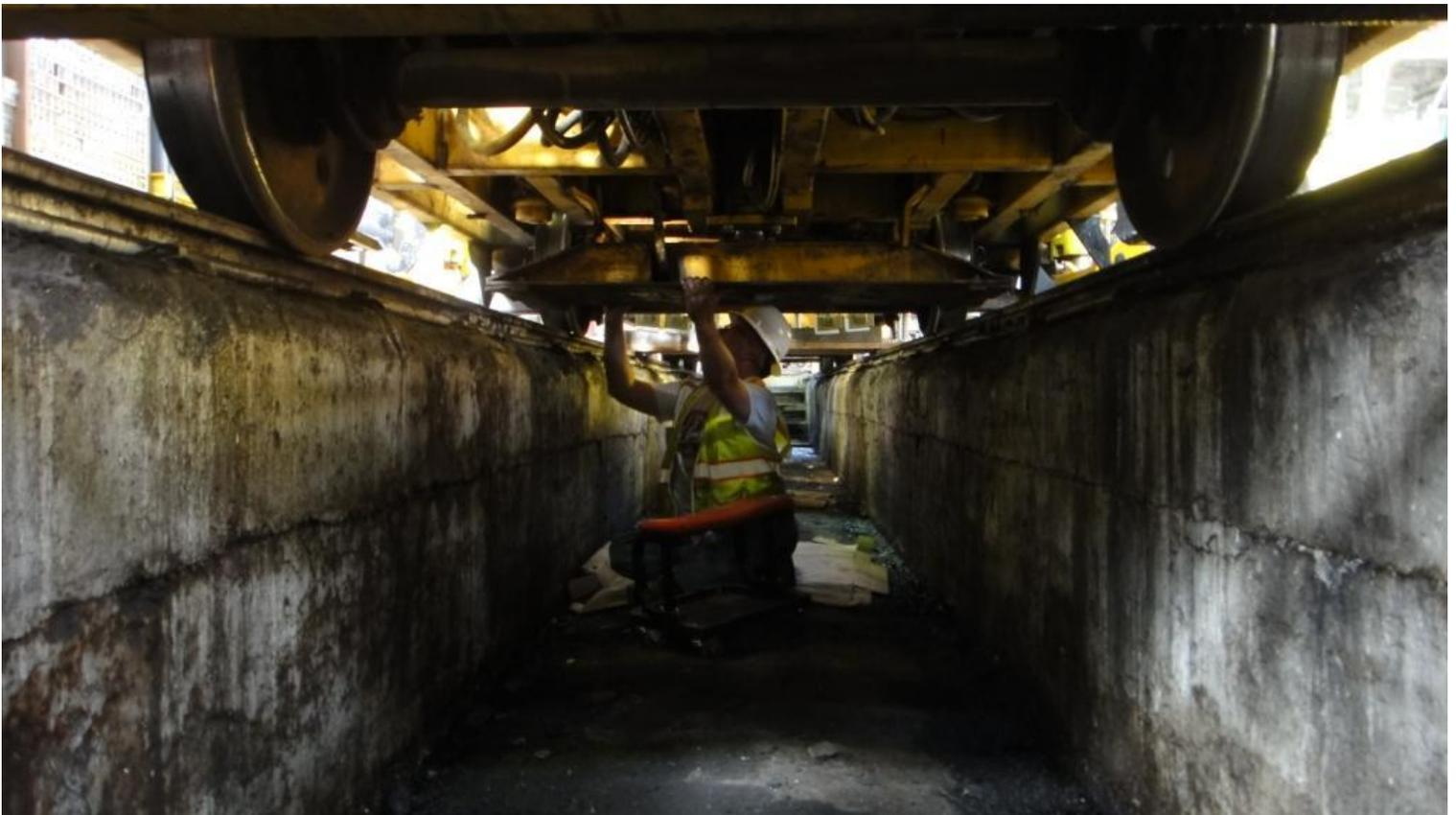
Scott in the pit under the new-old tamper to try to figure out why it has no "umph" in second gear
