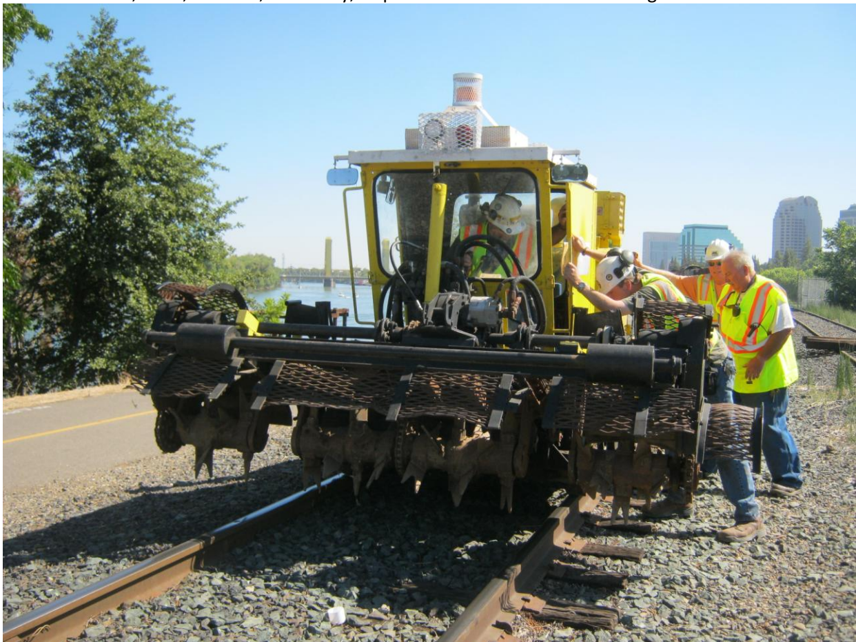
Using the scarifer's turntable to turn it around for its journey back to town.
