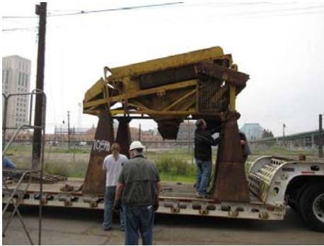
Loading the shaker on the truck for transport.
