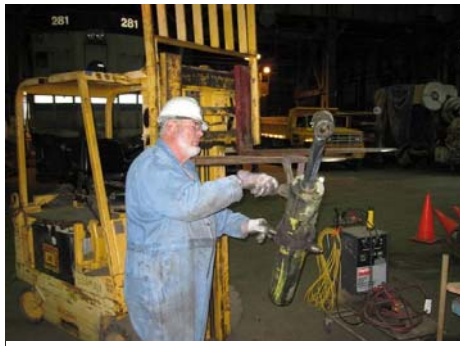
Sandy Cleaning up the lift cylinder from the Green Machine
