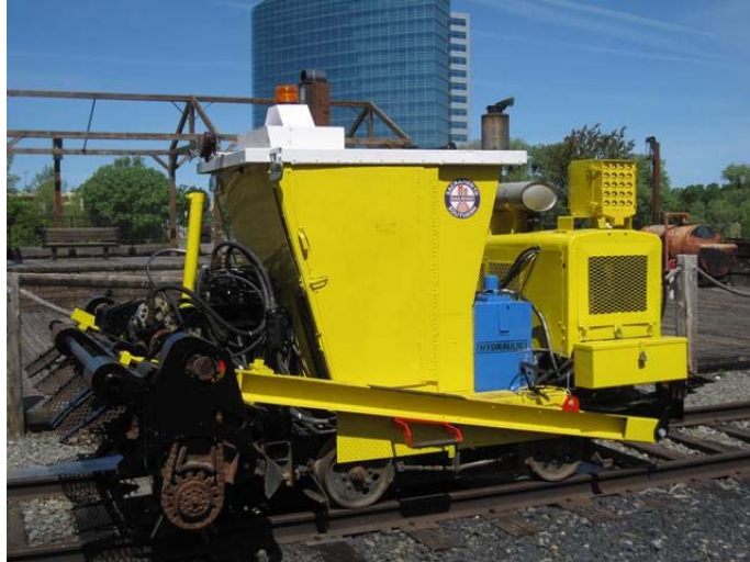
The Scarifier fresh out of the shop and ready for action. New teeth, engine service, horn repair, electrical repair, lube job, and new paint.
