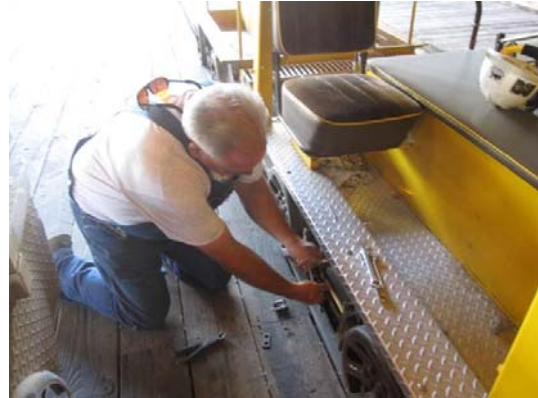
Harry adjusting the brakes on the interpretive motorcar.
